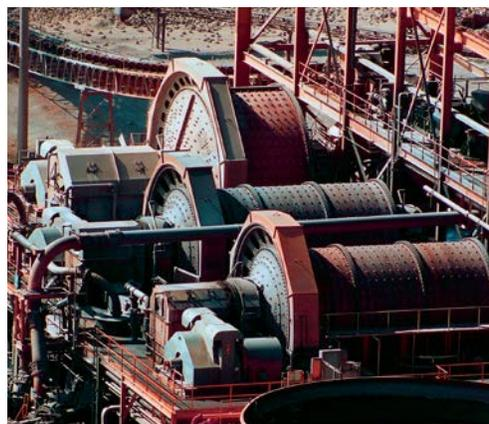
**SE55 Torque Limiters are designed to protect drivetrains from power spikes, jams and short circuits in high-torque applications, including mine ball and SAG mills.**
